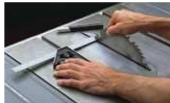
Next, slide the square and rotate the blade backward until the marked tooth aligns with the square. If the square just touches the side of the tooth, the slot and the blade are aligned.
