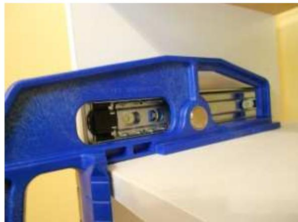
4. Once the jig is in position, drive the screws into the holes provided on the slide.
