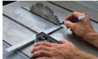
To check that your blade is parallel with the miter gauge slot, first mark a tooth. Then, place a square in the slot and adjust it so the end of the square just touches the side of the marked tooth.
