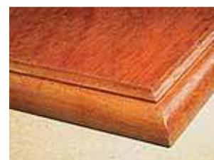
In the bottom photo, the face is sanded with 220-grit and the end grain with 600-grit, resulting in a much better color match.
