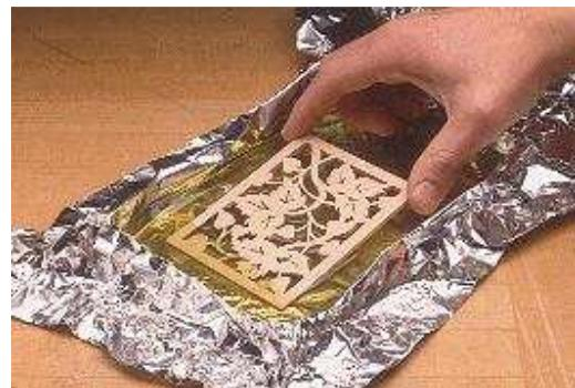
As for applying a finish, get into the tiny openings by dipping the panel in an oil finish, see photo. When dipping a fretwork panel, aluminum foil shaped into a tray acts as a reservoir for the oil finish. To remove the excess finish, you can blot the panel dry with a cloth or blow it out with compressed air.
