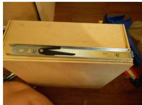
6. For inset drawers, you will need to mark the inside of the cabinet where the slides will be located. Make a mark of 3/4" in from the front edge.\
