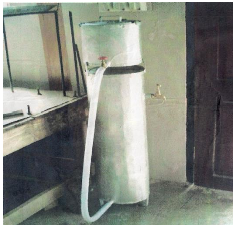
Figure 61: Domestic water filter (Bolaji et al. , 2010b).
