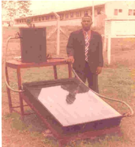
Figure 10. The experimental set-up of the solar water heating system (Source: Bolaji, 1993)
