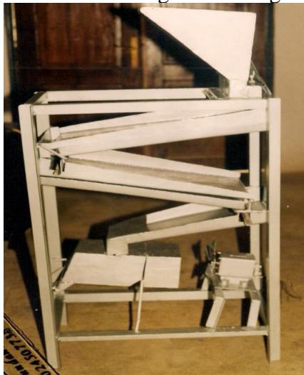
Figure 64. Rice de-stoning machine (Adejuyigbe and Bolaji, 2012)
