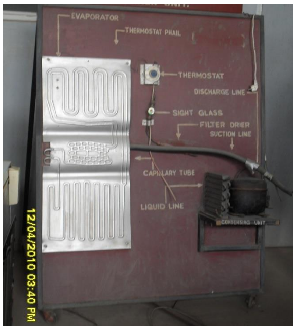
Figure 66. Apparatus for demonstrating vapour compression refrigeration system (Bolaji and Falade, 2012).
