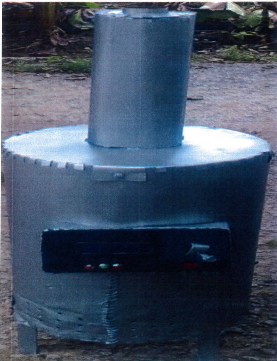
Plate 4.1 The designed and fabricated steam boiler
