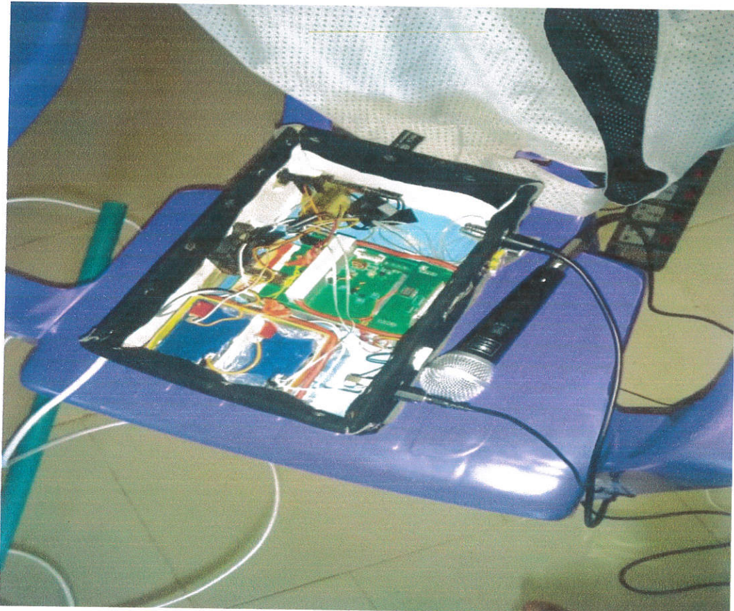
Fig 4.1: Internal arrangement of the mini-broadcast transmitter.
