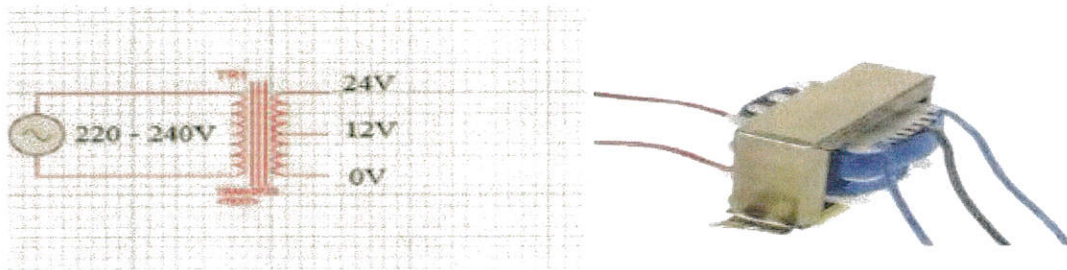
Figure 3.5 Showing Step down transformer
