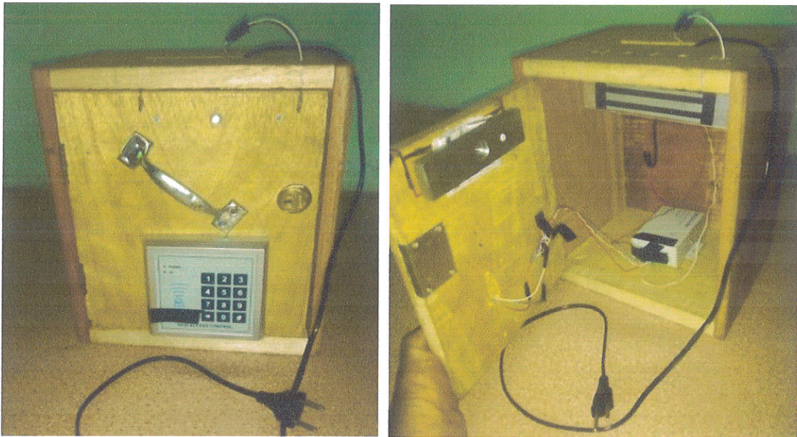
Figure 4.6: The prototype of the microcontroller based door access control using radio frequency identification
