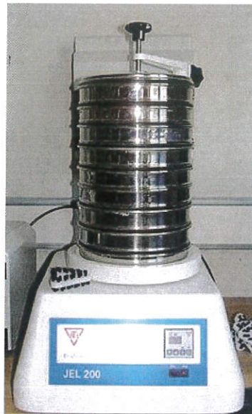
Fig. 3.2: A mechanical shaker used for sieve analysis.
