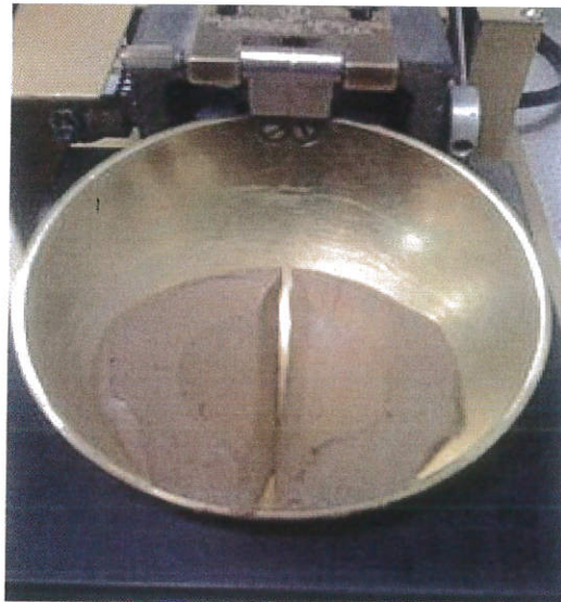
Fig. 3.3: Casagrande cup in action
