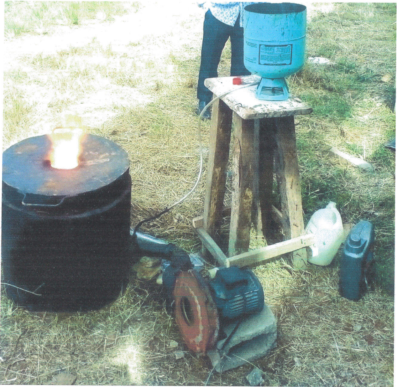
Plate 4.2: Layout of the constructed Furnace during Testing
