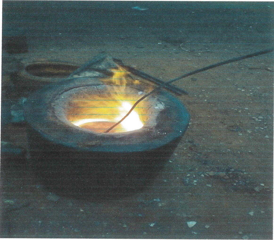
Plate 4.3: A Picture of the Furnace During the Removal of the Melt from the Furnace
