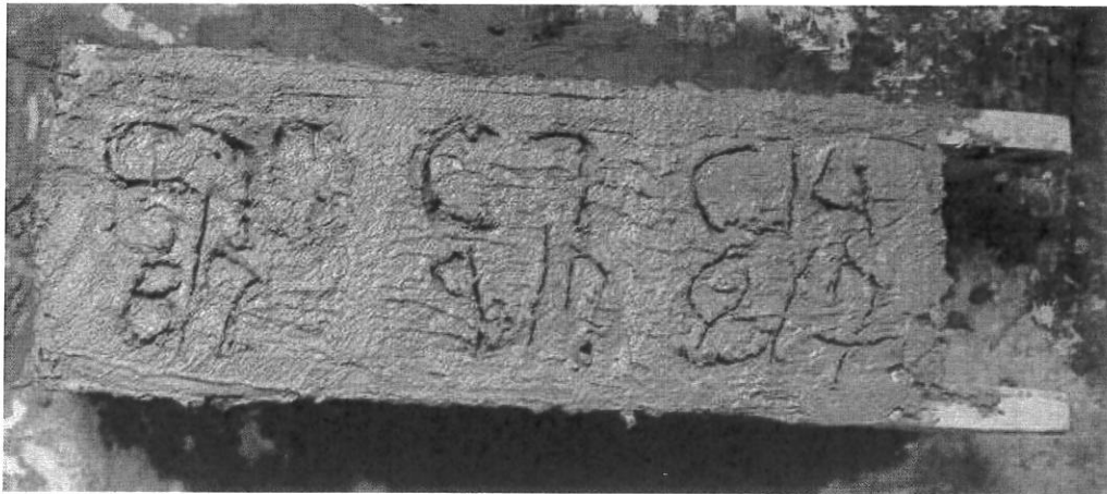
Plate 3.10 Labelling concrete cube
