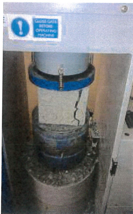
Plate 3.13 Failure occurring to cube during Crushing
