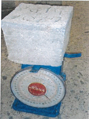
Plate 3.11 Weighing of Concrete cube
