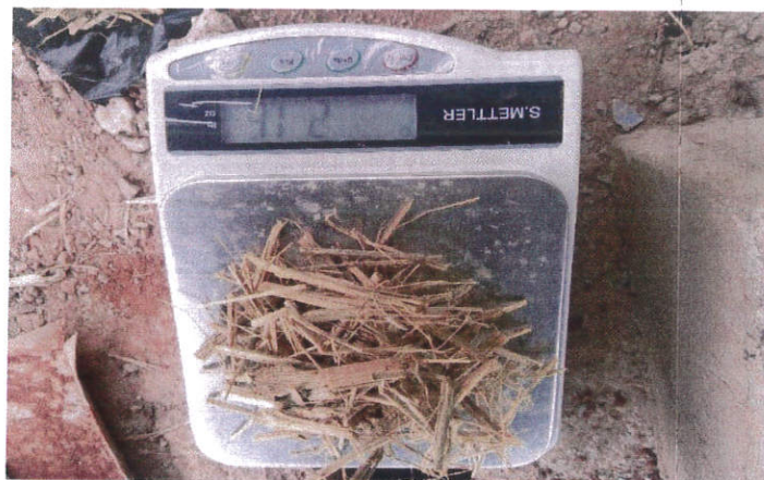
Figure 3.4: Weighing of Fiber for Composite Preparation
