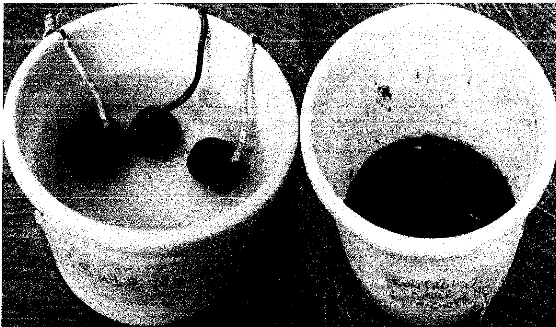
Plate 3.8: Appearance of Samples 1, 4, 7 and 11 in 3.5 wt% NaCl after 30 days
