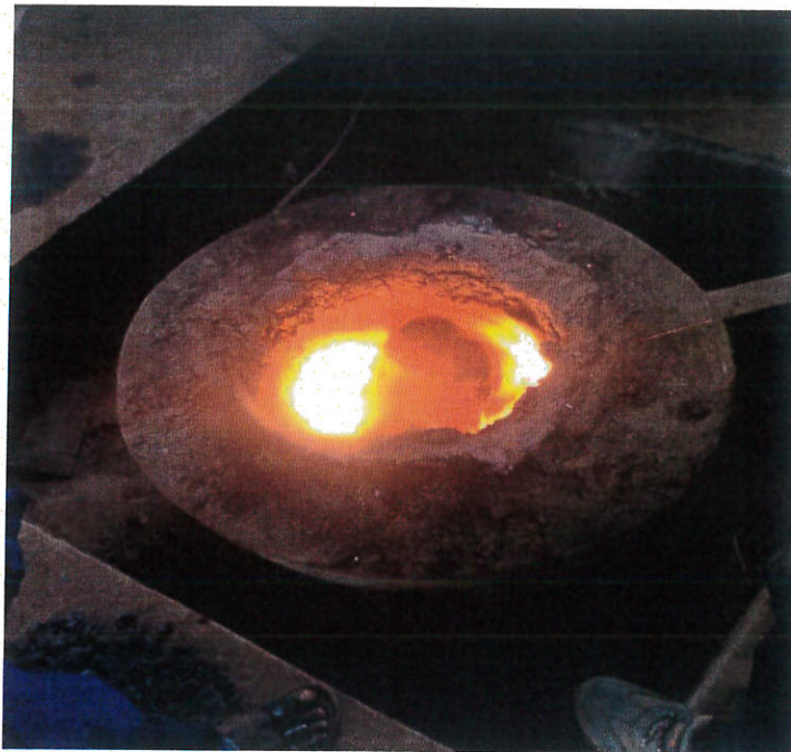
Plate 3.3: Pit crucible furnace
