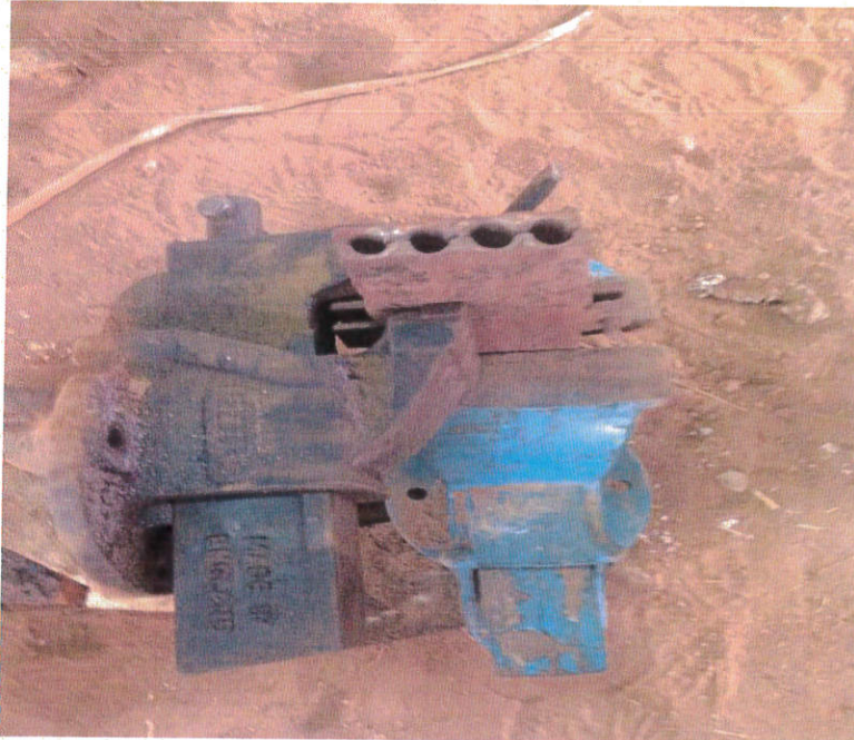
Plate 3.4: Bench vice holding the metal mold firm
