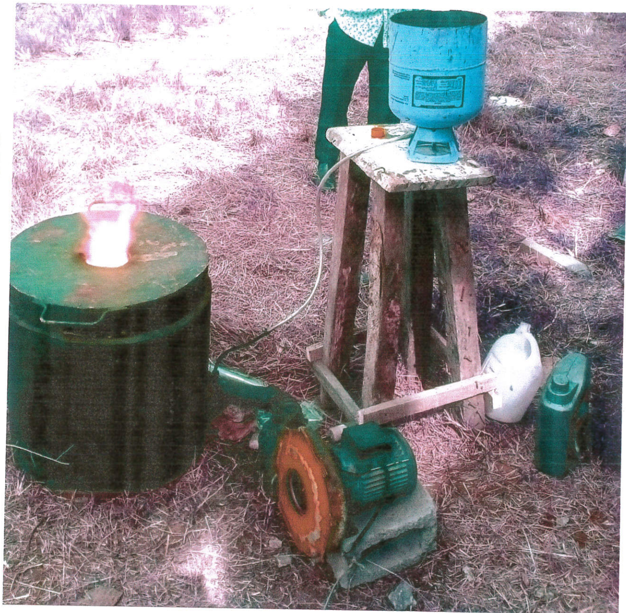
Plate 4.2: Layout of the constructed Furnace during Testing
