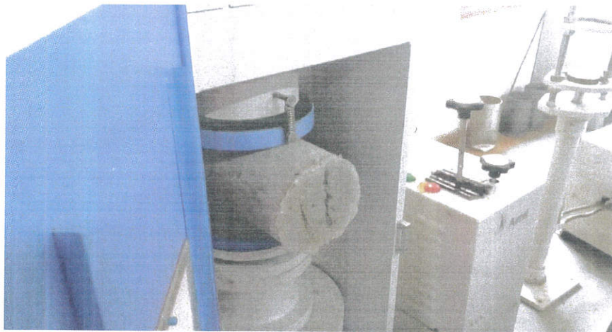
Plate 3.19: cylindrical specimen under the application of load for tensile strength
