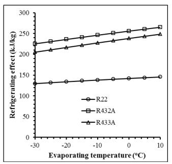
Fig. 3 Influence of evaporating temperature on the refrigerating effect
