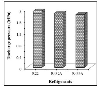
Fig. 8 Discharge pressure of the refrigerants at condensing temperature of 50°C
