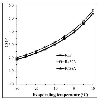
Fig. 10 Influence of the evaporating temperature on the coefficient of performance (COP)
