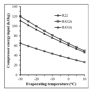
Fig. 4 Compressor energy input versus evaporating temperature
