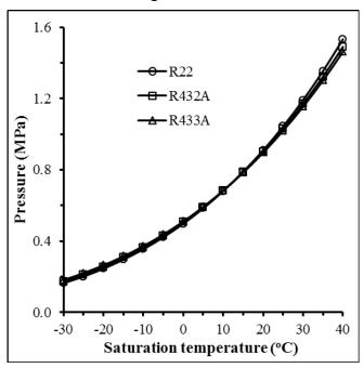
Fig. 2 Saturation vapour pressure curves
