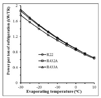
Fig. 5 Influence of evaporating temperature on the power per ton of refrigeration
