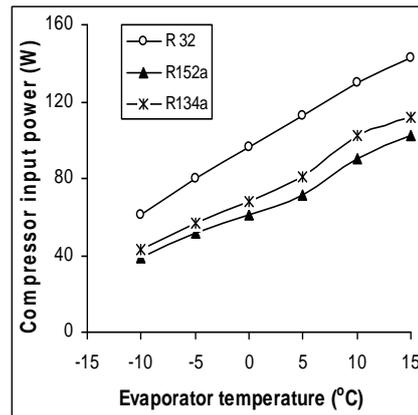
**Figure 7.** Variation of compressor input power with varying evaporator temperature for R32, R152a and R134a.
