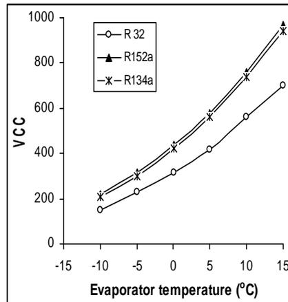
**Figure 8.** Variation of volumetric cooling capacity (VCC) with varying evaporator temperature for R32, R152a and R134a.
