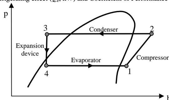
**Figure 1.** Vapour compression refrigeration system on p-h diagram.
