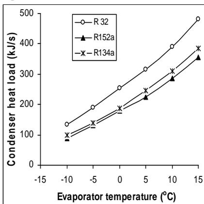
**Figure 6.** Variation of condenser heat load with varying evaporator temperature for R32, R152a and R134a.
