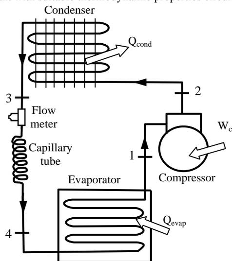
**Figure 2.** Schematic diagram of a vapour compression refrigerator.
