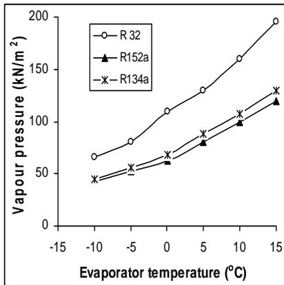
**Figure 4.** Variation of vapour pressure with varying evaporator temperature for R32, R152a and R134a.
