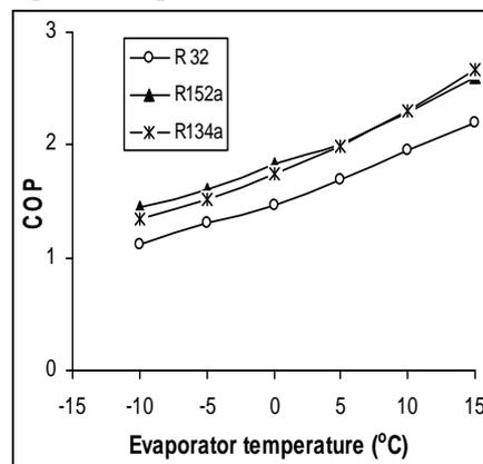
**Figure 9.** Variation of coefficient of performance (COP) with varying evaporator temperature for R32, R152a and R134a.
