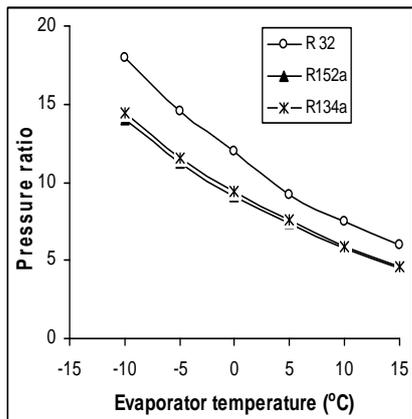
**Figure 5.** Variation of pressure ratio with varying evaporator temperature for R32, R152a and R134a.
