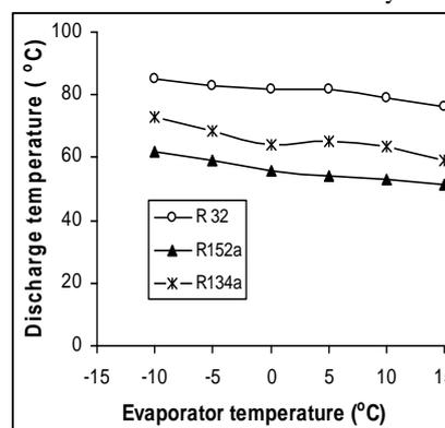
**Figure 3.** Variation of discharge temperature with varying evaporator temperature for R32, R152a and R134a.
