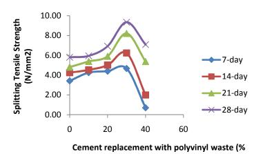
*Figure 9: Effect of Polyvinyl Waste on the Splitting Strength of the Specimens*
