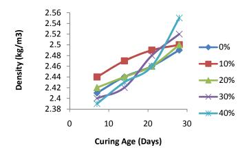
Figure 6: Variation of Density of Concrete incorporating Polyvinyl waste powder (PWP) with Curing Age
