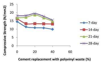
*Figure 8: Effect of Polyvinyl waste powder (PWP) on the Compressive Strength of Concrete*
