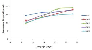
*Figure 7: Variation of Strength with Curing Ages for Concrete incorporating Polyvinyl waste powder (PWP)*
