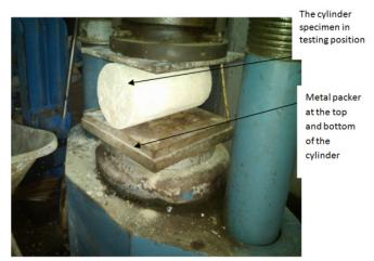
Figure 1: Splitting Test Specimens
