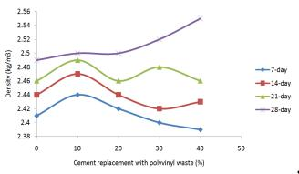
*Figure 5: Effect of Polyvinyl waste powder (PWP) on the Density of Concrete Specimens*
