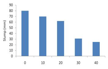
Cement replacement with polyvinyl waste (%) Figure 4: Effect of Polyvinyl waste powder (PWP) on the Workability of Concrete
