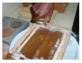
Figure 4: Sample tested for water penetration
